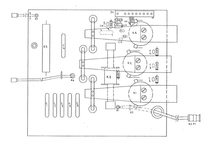
Figure 10-1. RF Output PCB Assembly A4, Component Locations
