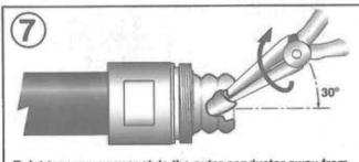
Twist-tear can opener style the outer conductor away from the dielectric. Tear at an angle, rolling against the spring fingers forming a flared contact against the fingers.
