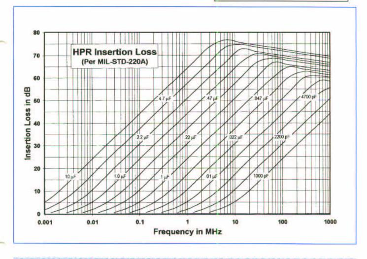
Patented HPR for high frequency and high current.
