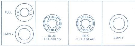
The Vuemaster Liquid Indicator: Reads "FULL" when the system is fully charged. It remains blank when there is a shortage of refrigerant in the liquid line.
