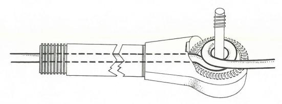
FOR INTERNAL FEED-THRU WIRING, WRAP ONE TURN OF MICROPHONE CABLE AROUND BOLT AS SHOWN ON ILLUSTRATION. RE-ASSEMBLE PARTS IN REVERSE ORDER AS REMOVED.
