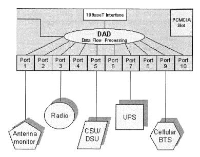
The SAM-10 uses Badger's Data Acquisition Device (DAD) software to collect serial alarm reports from the other network elements. The DAD software translates alarm and command data between the network elements and the Network Management System (NMS).
