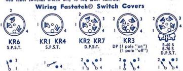
Note: All switch contact symbol views are with switch assembled to control and shaft in extreme counter-clockwise position.
