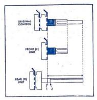
difficult-to-fit metal knobs, use a small "rat-tail" file to reduce the projections on inside of knob to allow knob assembly. A thin-nose pliers may be used to carefully rip or peel metal to the scored line on the shaft for use with double or single slot knobs. Burred edges must be filed smooth before assembly of front and rear controls.
