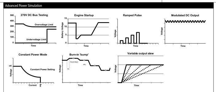
SGI model provides constant power mode allowing independent setting of the max voltage, current and power
