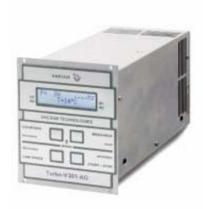
The Turbo-V 301-AG Rack controller is a microprocessorcontrolled frequency converter with new, enhanced features that allow greater control and communication capabilities. This compact, 1/4 rack unit is designed for full worldwide compatibility, for vent valve control, active gauge pressure reading and pump operation parameters control, as well as for self diagnostic and protection features.
