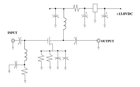
Schematic shown is the 13 dB gain, +30 IP3 output model.
