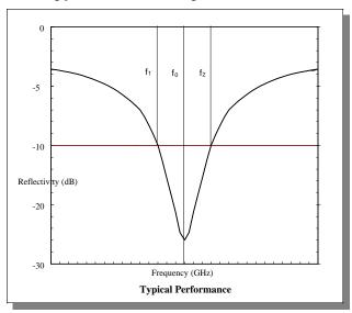
The performance of ECCOSORB® SF is defined by reflectivity at a single frequency. A generalized performance curve is shown above. The design frequency  $f_0$ , has a  $\pm 5\%$  bandwidth, designated as  $f_1$  and  $f_2$ . Although performance degrades with increased incidence angle, at incident angles out to  $45^\circ$ , reflectivity of -16dB has been demonstrated.
