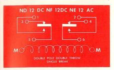
Time delay starts when coil is energized—control circuit closed
