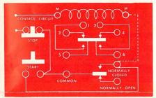
Dotted line represents jumper wire connected between "M" (coil) and N.C. contact of the microswitch when electrical interlock is desired. For models NEL-11, NDL-11, NFL-11. Also available in double pole.
