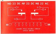
Time delay starts when coil is de-energized—control circuit opened
