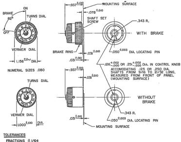
TYPICAL MOUNTING OF DIALS TO BUSHING MOUNT POTENTIOMETERS WITH 1/8 AND 1/4 SHAFT DIAS ON PANELS I/I6 AND 3/I6 THICK
