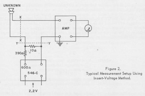
the Microvolter dials to produce the same deflection on the external meter as noted before. (The Microvolter should be operating with an input of 2.2 volts.) With the impedance values shown in the diagram, the unknown voltage will be  $\frac{10}{600+390+10}$  or 1/100 of that indicated on the Micro-
